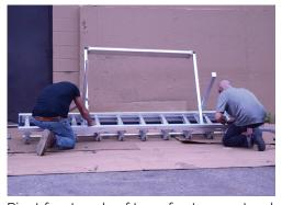
Pivot front ends of top of extreme stand into front brackets and secure with fast pins.
