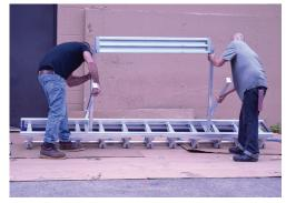
Insert back ends of top of extreme stand into rear brackets and secure with fast pins.
