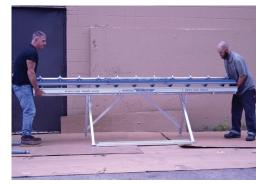
From the rear of the brake, remove fast pins from rear struts on base rails of brake and lower struts to meet rear legs of extreme stand. Insert fast pins to secure struts in place.
