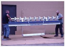
Use two people to lift brake and set up in normal operating position and pivot walk board at front of stand into flat position.
